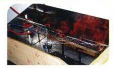
Category Z - Exposure to Fire with Mechanical Shock at 950° C as per BS 6387
